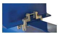
STEP 3 - Once the sections are in the desired position, tighten each clamping screw to the recommended torque of 20Nm (15 ft/lbs)
